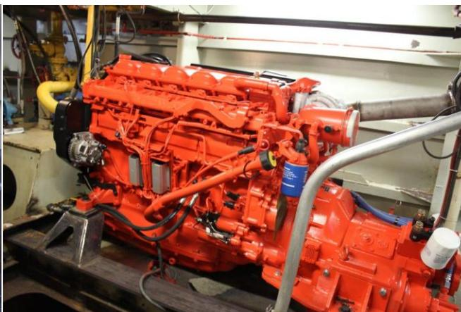
***One of two new Scania 400hp high efficiency diesels***
