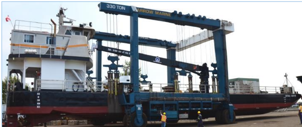
90’ of New Hull/Deck – includes a 30’ increase in length overall (120’ to 150’)
