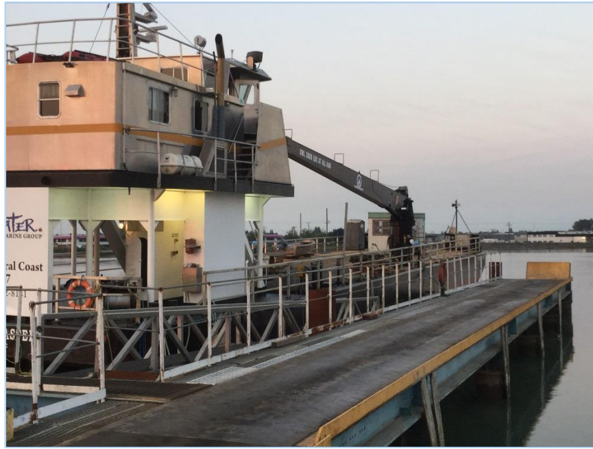
A 15-ton capacity Seven Stars Pedestal Crane with 70' boom – greater reach and load.
